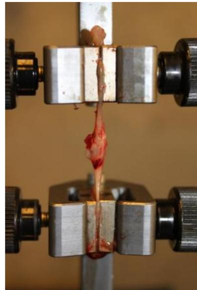
The anastomosis is pulled apart at a constant speed of 10 mm/min.
